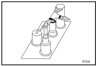
Fig. 50 Correct pilot flame pattern. PSE Pilot.
